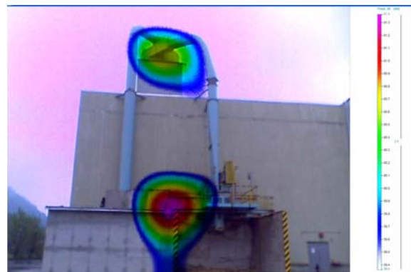
Fig. 5: Visualization of the noise emission intensity
